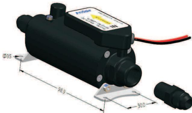
Within the body of the PX375-TC Boost Pump is contained the Bypass. This feature allows for fuel to flow around the positive displacement pump, whilst the pump is not running. The porting within the body has been computer optimised to ensure the best possible flow conditions.
